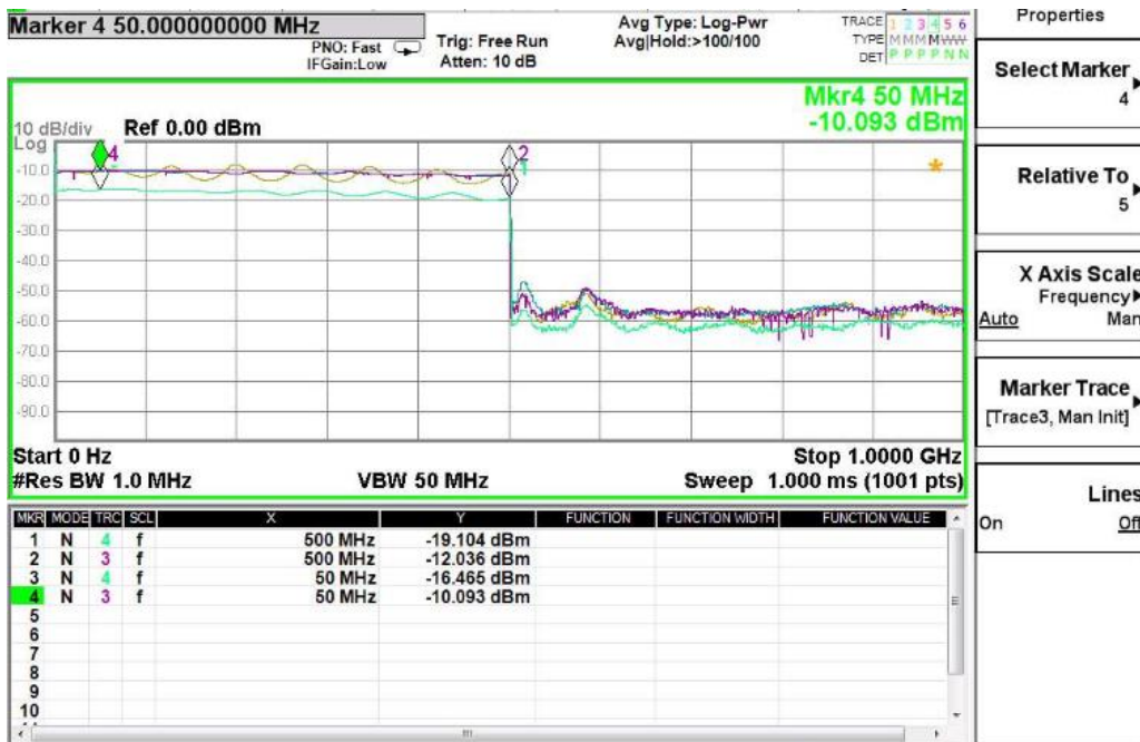
Fig. 4 – Combiner performance Trace 1 and 3 as input Trace 4 is output
